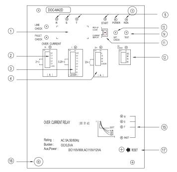
1. Current Display / Operating Count 2. Curr. Limits Element 3. Time Lever Element 4. Instantaneous Element 5. R - Phase Indicator 6. S - Phase Indicator 7. T - Phase Indicator 8. Over current Start Indicator 9. Power Lamp LED 10, CPU Run Indicator 11. Monitor Selection Switch 12. Time curve Selection Switch 13. Setting Check 14. Test 15. Fault Indicator 16. Draw - out Handle 17. Reset Button
